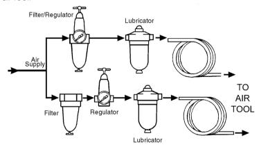
A typical air line layout is shown above. If an automatic in-line filter/regulator is used, it will keep the air tool in good condition, but should be regularly checked.
